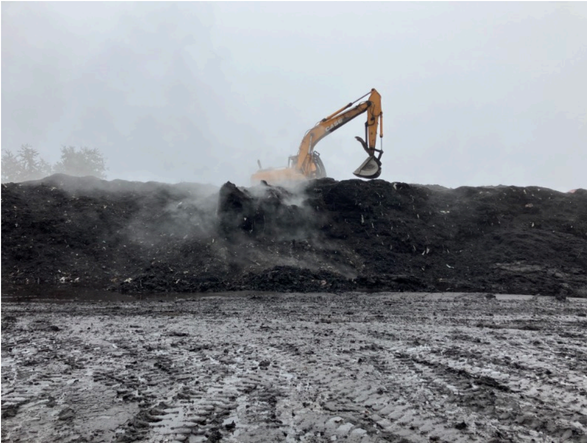
Photo 1. Run-off water collecting around the compost pile at the storage site with no leachate control.
