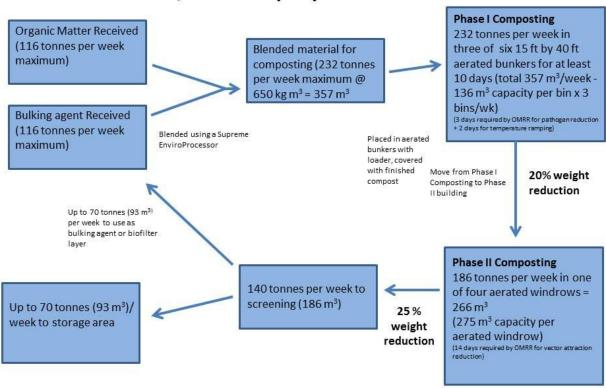
This design meets the requirements for the BC Organic Matter Recycling Regulation (OMRR), which requires a potential pathogen reduction process (> 55 C for a minimum of three days – OMRR Schedule 1) and a vector attraction reduction process (>14 days under aerobic conditions at average temperature > 45 C – OMRR Schedule 2).
