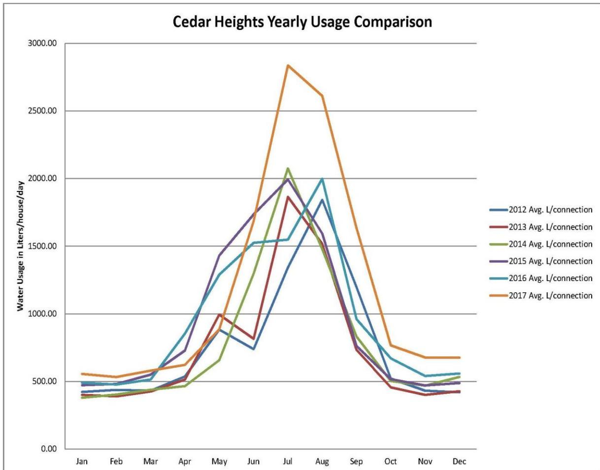
The CSRD has a water flow meter at its intake and the yearly pumping total and monthly pumping total are illustrated in the following graphs.
