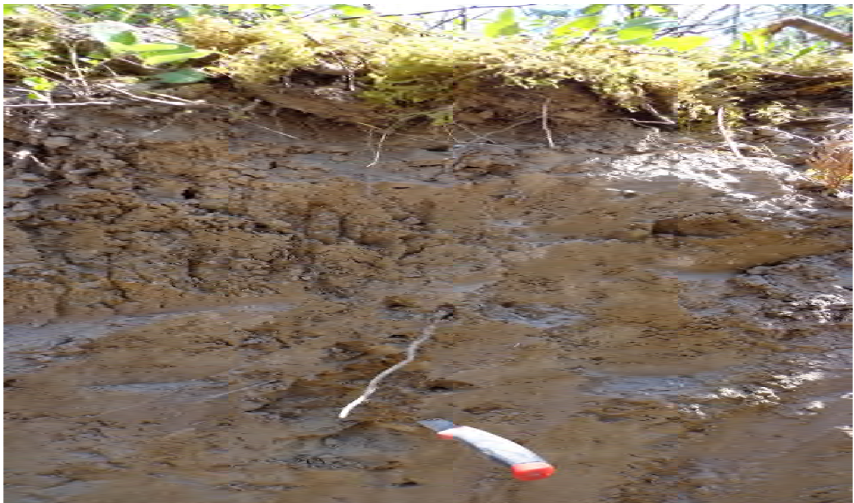
Photo #4. Soil test pit TP4 an Orthic Gray Luvisol with heavy clay over deep sand.
