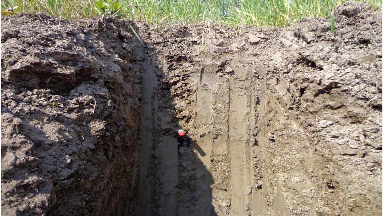
Photo #1. Soil test pit TP1 an Orthic Gray Luvisol with heavy clay in the Bt.
