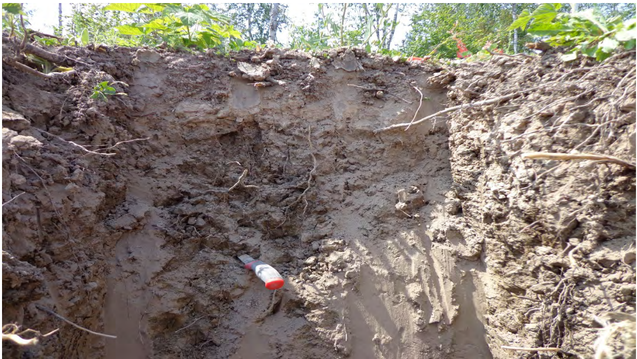
Photo #2. Soil test pit TP2 an Orthic Gray Luvisol with heavy clay in the Bt.
