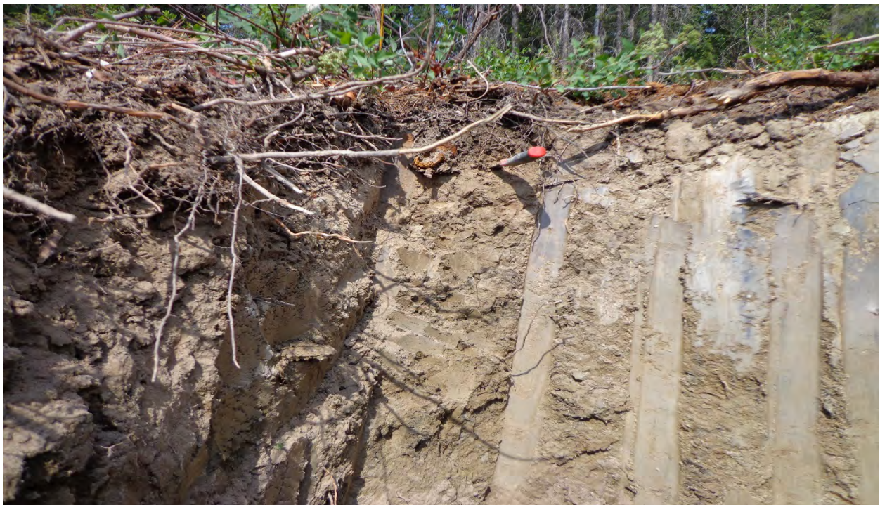
Photo #6. Soil test pit TP6 an Orthic Gray Luvisol with silty clay in the Bt.
