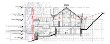
Please see the attached site sections, which illustrate the height of the proposed principal structure relative to the steep bank to the southwest, as well as the lower elevation of the deck supports due to the sloping nature of the site. The included elevation details further support our design rationale, emphasizing the careful consideration given to the unique topography and the effort to maintain a cohesive and naturally integrated structure.
