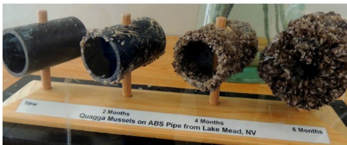
This photo shows how quickly quagga mussels have colonized on pieces of pipe in Lake Mead (Nevada) over different periods of time. This imposes very costly ongoing maintenance to rid pipes and other infrastructure of mussel colonies.
