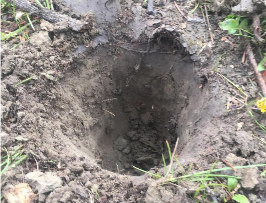
**Photo 3** Soil profile on the property consisting of firm SILT some fine sand
