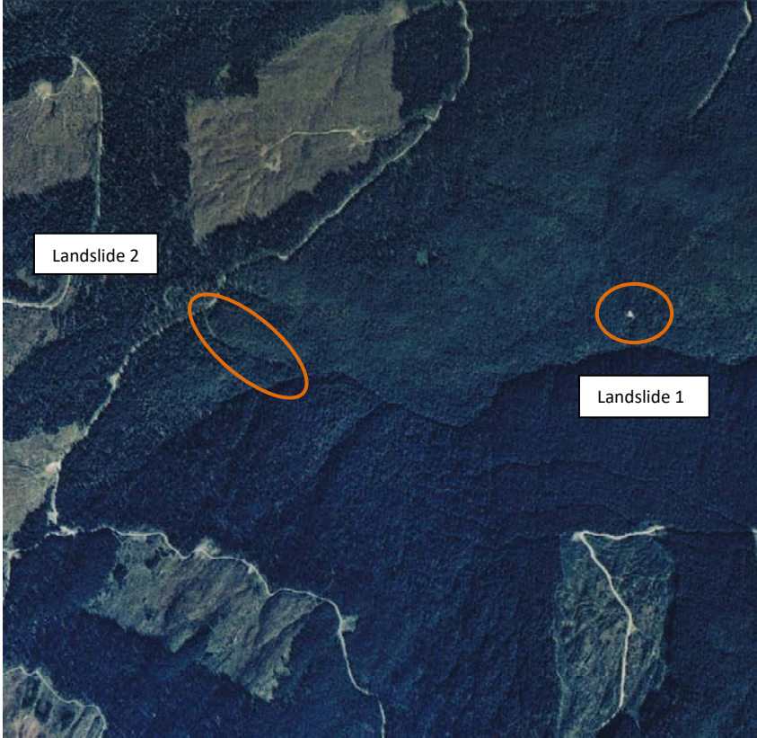
Photo 9 – 2001 airphoto of study area. Landslide 1 and 2 are visible but Landslide 3 appears to have fully revegetated.
