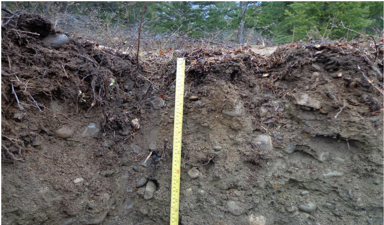
Photo#4. Close-up of TP1 showing the brown Bm (4-23) horizon in the upper soil.
