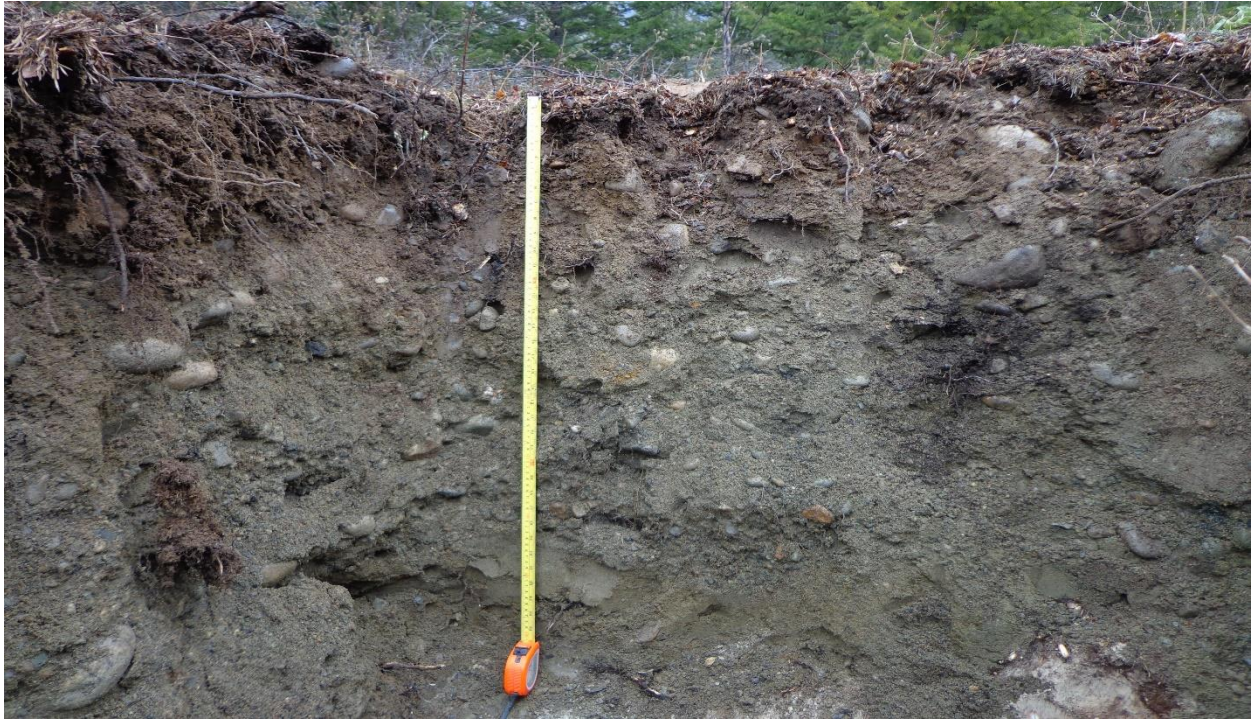
Photo#3. Soil test pit TP1 located next to the NW corner of the footprint on undisturbed land.
