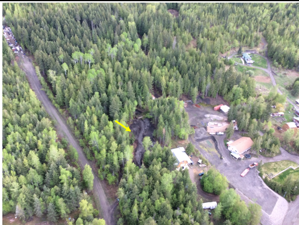
Photo 2 – View looking south at the bank instability and channel disturbance (arrow) within the east tributary creek south of (above) Taylor Road and west of Hannett Road (the road on the left side of the creek). [May 9, 2018]
