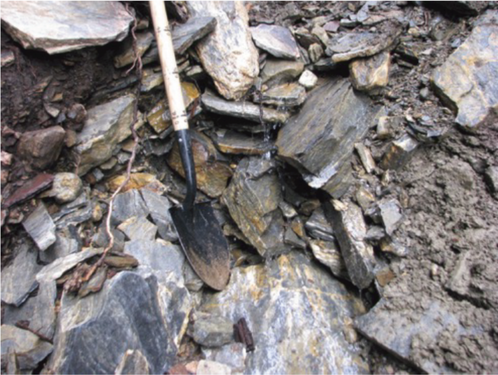
Photo 12 – View of the coarse angular fragments in the gully channel, in the lower part of the initiation zone. The gradation on the shovel is 10 cm. A spring was emerging from the coarse sediment. Photo was taken on May 15, 2017.
