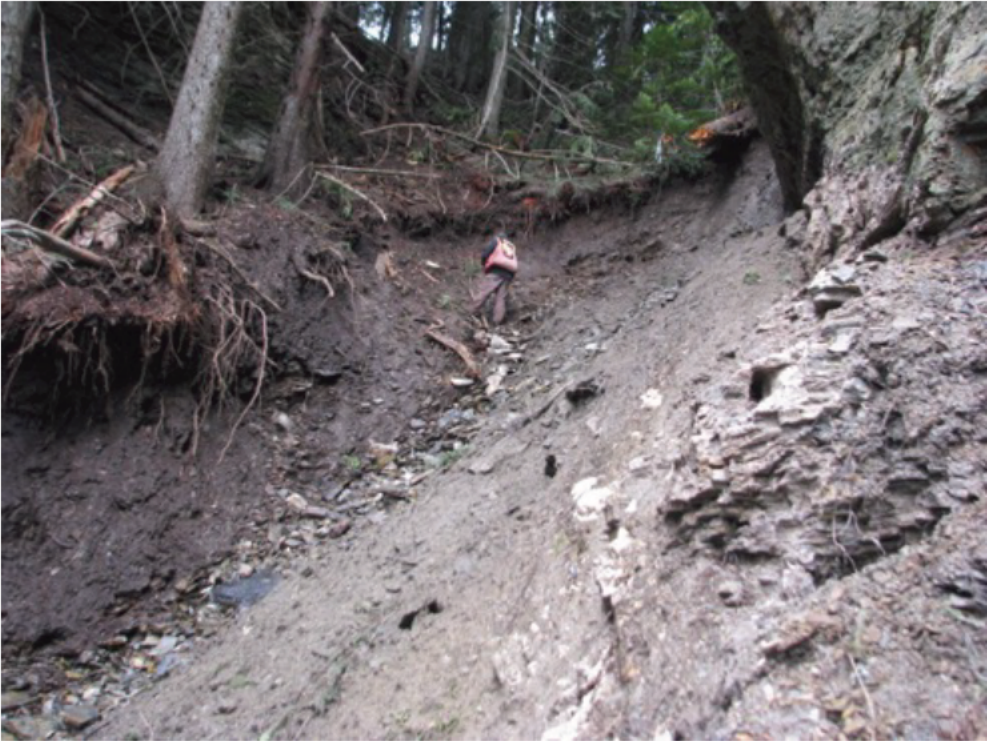
Photo 9 – View up to the scarp taken on May 15, 2017. Note the bedrock present on the right side of the photo, which extends up a high cliff to the plateau edge. A stream emerges from the rubble below the person. Tension cracks were observed to the left behind the tree (Photo 11).
