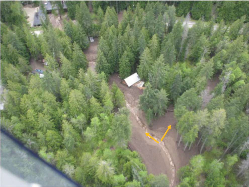
Photo 5 – View downstream of the residence on 5921 Sunnybrae – Canoe Point Road that was destroyed on May 6, 2017. The debris flow bifurcated as shown and a small lobe of debris travelled through the trees to the right.
