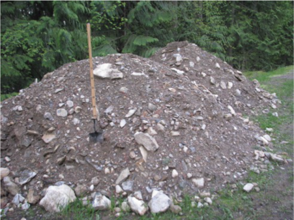
Photo 24 – View of the typical fan material that was piled up on the public road shoulder from a local excavation. It shows the gradation of the material. A gradation analysis on the minus 75 mm fraction of the debris deposit is attached in Tab 4.
