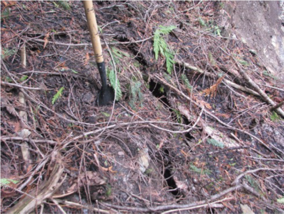
Photo 11 – This photo shows tension cracks that had formed in the colluvium on the right bank near the scarp. Photo was taken on May 15, 2017.
