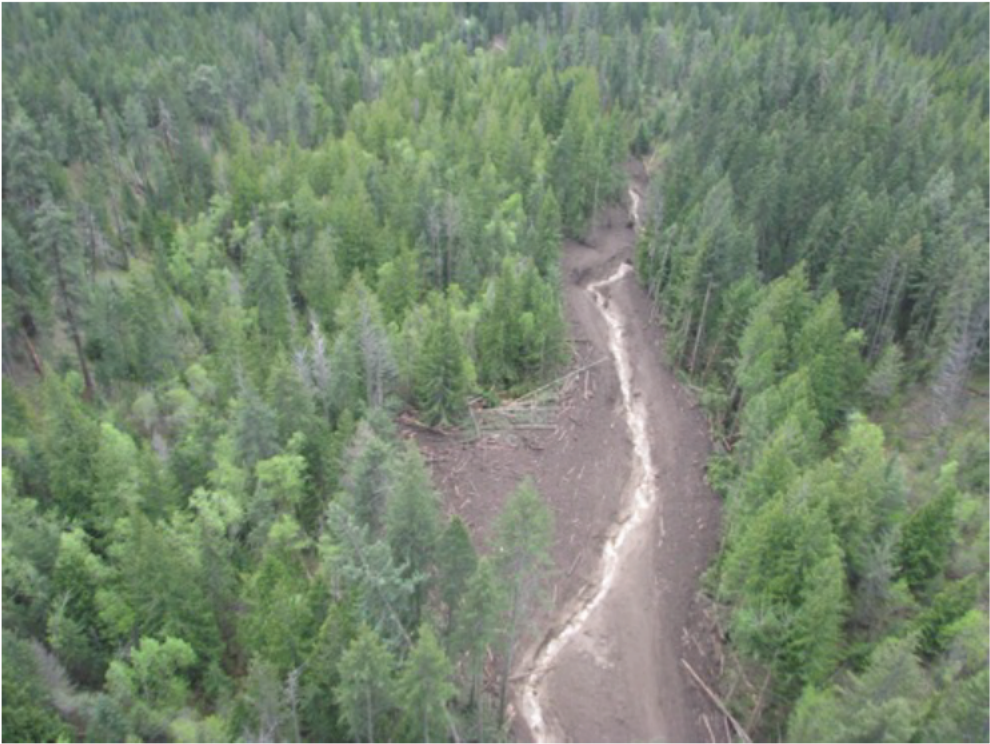
Photo 4 – View downstream (south) of the upper part of the logjam and debris deposit, just downstream of the fan apex. This deposit may have deflected the debris away from the east side of the fan.
