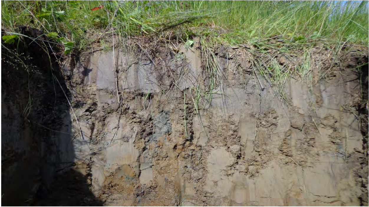
Photo #5. Soil test pit TP5 an Orthic Humic Gleysol with silt loam and prominent mottles.
