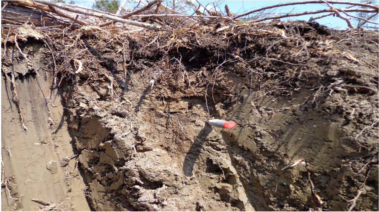
Photo #3. Soil test pit TP3 an Orthic Gray Luvisol with heavy clay over silty clay.
