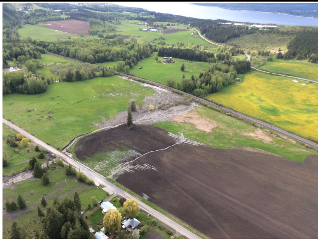
Photo 4 – View looking northwest at an area with considerable sediment deposition along the east tributary creek between London Lane (foreground) and the CP Railway. Deposition is visible upstream of London Lane in the left side of the photograph [May 9, 2018]
