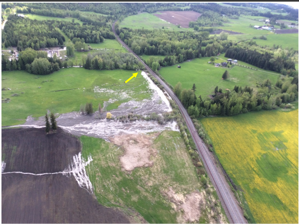
Photo 5 – View looking east over the sediment deposition above the CP Railway. At the time, the east tributary appears to have been partially diverted to the west tributary (arrow). [May 9, 2018]
